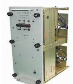
Multi Function Radar for Korean medium-range Surface-To-Air missile system Power Supply
