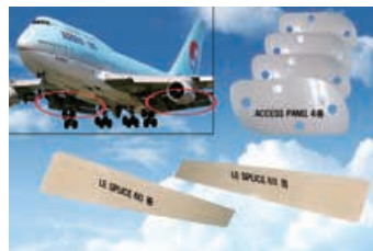
LE Splice and Access Panel
